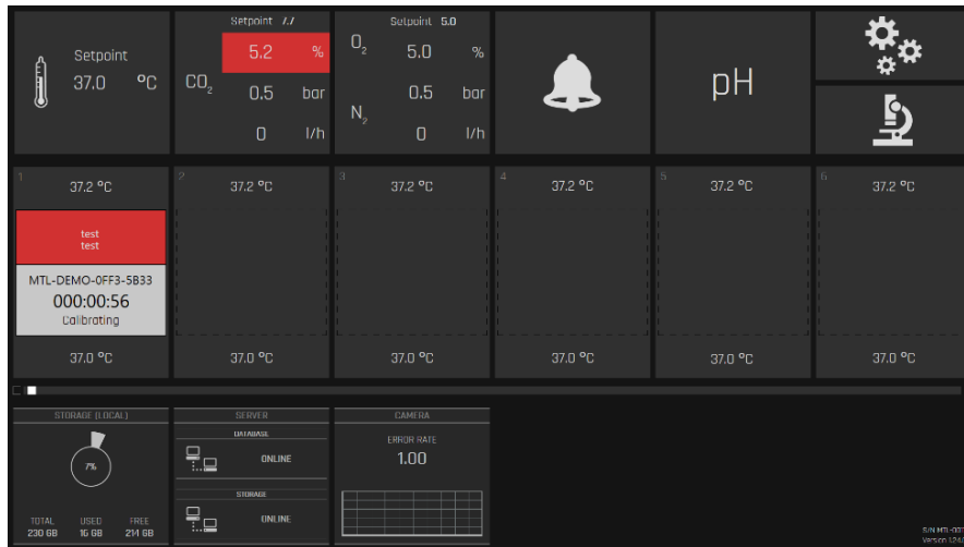
Figure 20.38 CO 2 concentration alarm view
